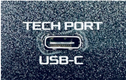
Firmware update is made via the USB-C connector.
