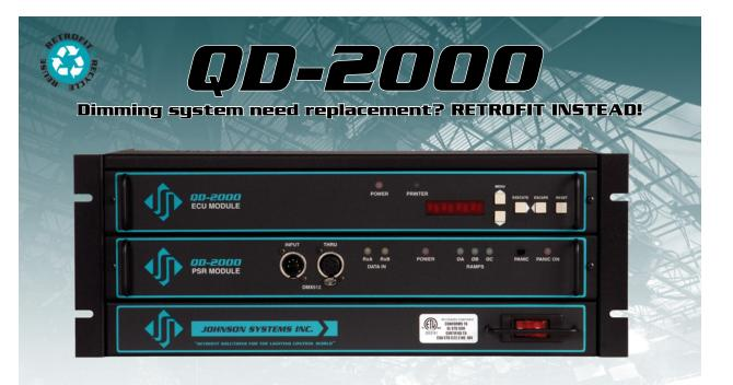
The QD-2000 is a professional retrofit electronics package designed specifically for Electro Controls (EC) Quad dimmer racks. This full-featured, state-of-theart unit converts dual DMX inputs with protocol manager to 96 PWM and 128 DMX channels of output. Standard software includes architectural features such as DMX snapshots, scene storage, time clock, power management, auto scheduling, dimmer rack diagnostics and much more.
